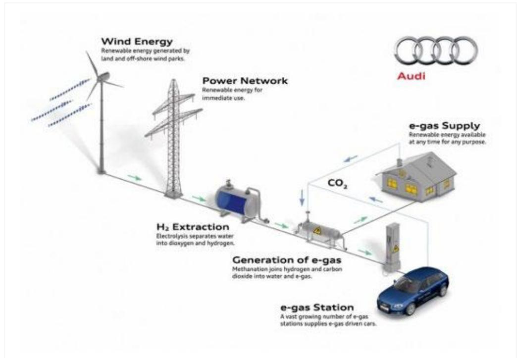
Other demonstration projects recently or currently being commissioned include the KIC-Project „DemoSNG“<sup>24</sup>, which uses biogas as a carbon source to produce 10 m<sup>3</sup>/h of renewable natural gas and the 1 MW BioCatProject<sup>25</sup>, which uses a biological methanation process as part of the Power-to-Gas process chain.
