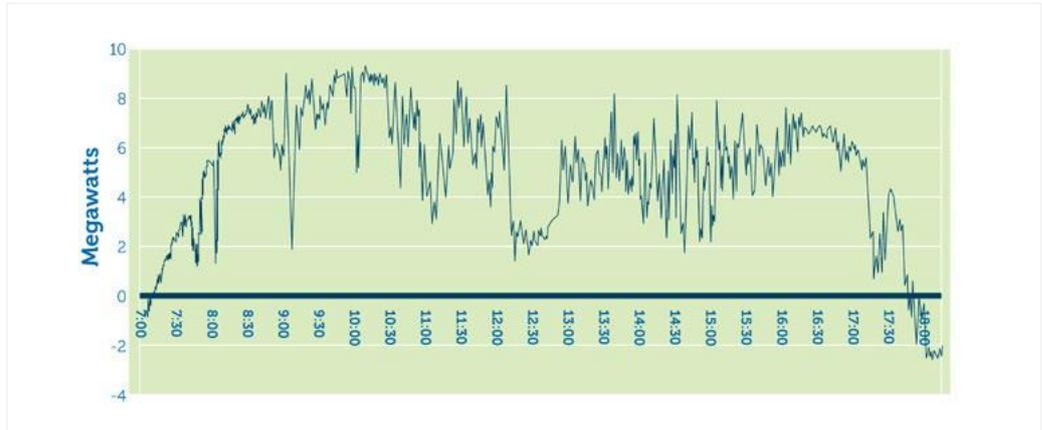
*Solar PV output on a partly cloudy day<sup>4</sup>*
